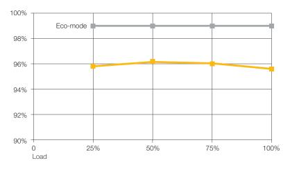
High efficiency reaching 96.1% Flat curve  $\rightarrow$  95.8% at 25% load
