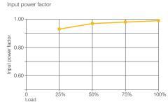
Near unity input power factor, at partial and full load, reduces the required size of the input cable and fuses, thereby reducing the materials (and costs) associated with the system's electrical installation.
